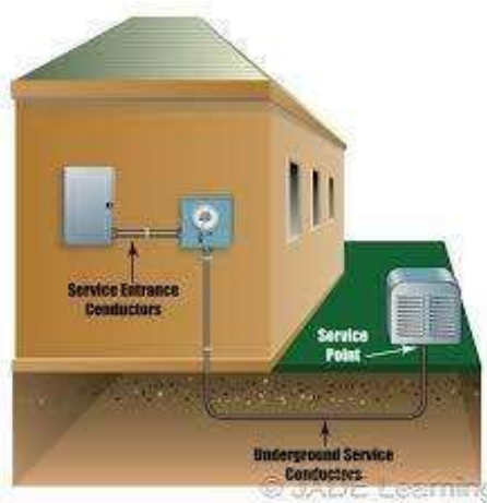
Typical Underground Service
